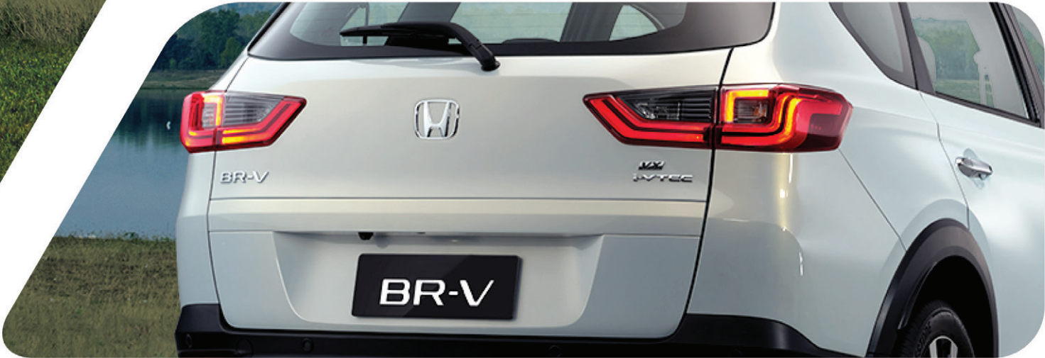
Rear Combination Lights (with LED Light Bars)
